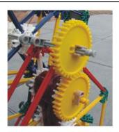
Two pupils have built a big wheel from K'nex (see the pictures above). The motor is attached to a gear that drives another gear (of equal size) on the axis of the big wheel. As a teacher you want to pose a question to encourage the pupils to formulate their own questions about cause-effect.
